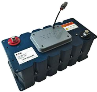
3. The XLR modules consist of 18 individual Eaton XL60 supercapacitor cells designed to provide 48.6 V and 166 F with 5 mΩ dc resistance for incorporation into systems requiring up to 750 V. (Courtesy of Eaton)
