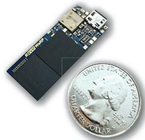
2. Revolution Robotics’ Warp_0x01 module is based on NXP’s i.MX6 SoloLite adding memory, 802.11b/g/n WiFi, Bluetooth Low Energy 4.0 and a six-axis sensor.
