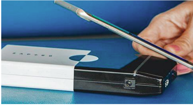
2. Zap&Go allows you to charge up to three devices simultaneously, two using the twin USB 2.0 ports and the third using the Qi wireless charging disc. (Courtesy of IEEE Spectrum)
