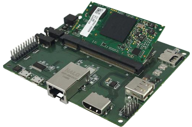
7. This carrier board was designed using the web-based Geppetto from Gumstix.
