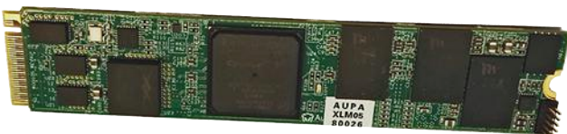
1. Aupera's M.2 module uses Everspin's 256 Mbit MRAM chips to provide storage that is faster and has a longer write lifetime than any NAND solution on the market.
