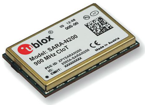
1b. The SARA-N2 module is u-blox's new NB-IoT module. Its package is 16 x 26 mm.
