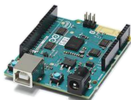
1. The Arduino 101 board runs Intel’s Curie chip with a 128-node neural network supported by General Vision’s CurieNeurons library.
