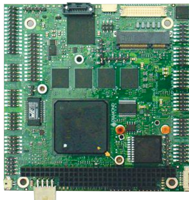
3. Diamond Systems' Helix allocates almost half the board to connectors, including the PC/104 ISA and a Mini PCIe socket.
